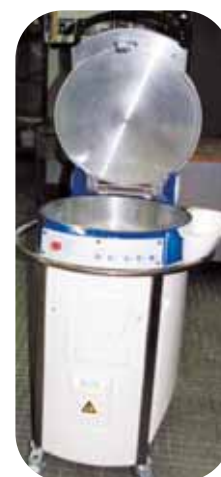
Diviseuse anti-projection de farine
